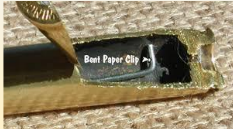
AMU 600 yard brass. Example over pressure loads
