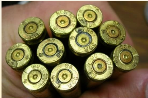
AMU 600 yard brass. Example over pressure loads
